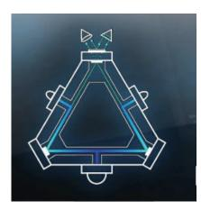
Optical technologies RLG & FOG sensing technologies form the basis of many of our motion sensors. Their role is to measure the rotation of a device in free space. Both technologies use a phase interferometry to achieve these rotational measurements. The RLG or the FOGs are arranged in a group of 3, and complimented with 3 matched accelerometers, to form a 6 Degree Of Freedom (DOF) inertial measurement unit (IMU).
